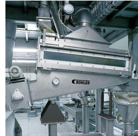
Air classification plant for production of legume protein concentrates
